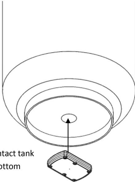
Rubber pad should contact tank
