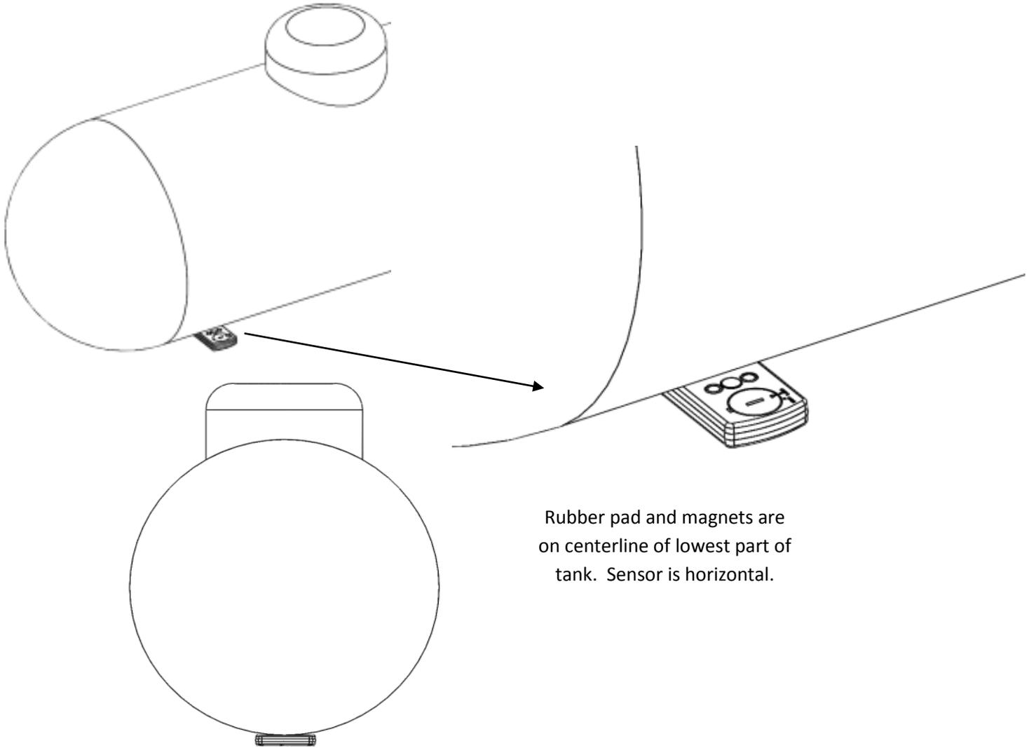
7. After a few seconds, up to a few minutes, the propane will settle and sensor readings will stabilize.
