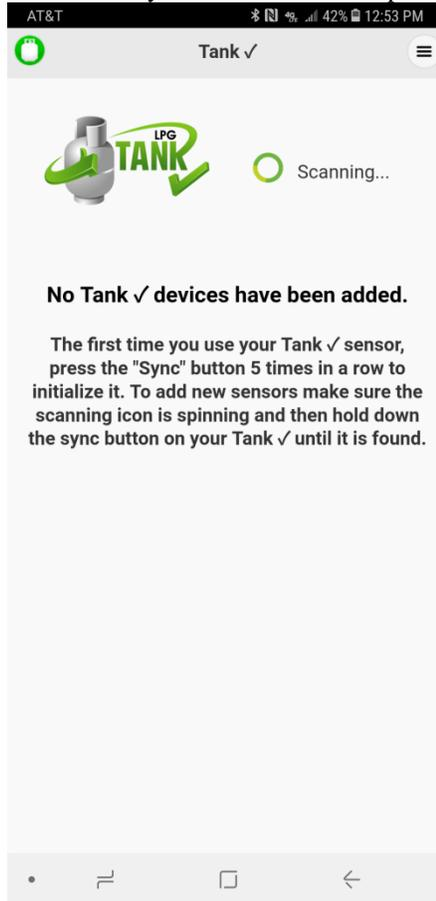
3. While the app is scanning, press the sensor SYNC button (Fig 1) a minimum of 6X quickly. *Note: The first 5X awaken the sensor from sleep mode. It is only in sleep mode from the factory. Once awake, the sensor will never go into sleep mode again; and only 1 press is required to re- SYNC or connect to a new device.*
