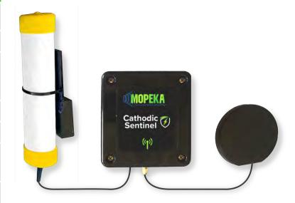
Mopeka® Cathodic Sentinel, the very first and only remote Cellular & Cloud Mobile Cathodic Protection. The Sentinel monitors the voltage, ground moisture level, and the current flowing from the tank to the anode bag(s) to validate that your tank is protected. It is safe, consistent, accurate, and reliable.
